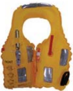
The Inflatable bladder is manufactured from high quality fabric (radio-frequency-welded yellow polyurethane coated nylon oxford buoyancy fabric) and inflation via a combined CO2 inflation manifold and oral inflation tube. As mentioned above, *the fabric is able to withstand 200,000 flex cycles without any physical damage.*
